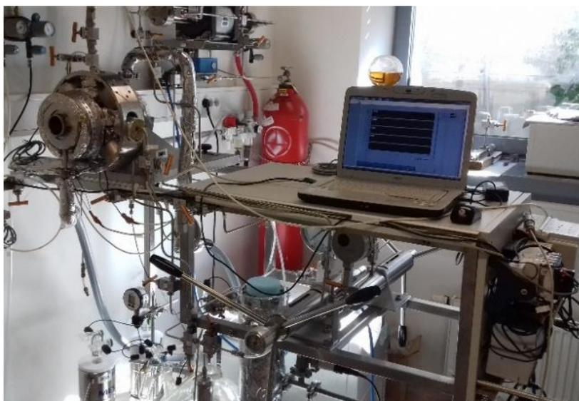
**Figure 1:** The apparatus for vapor-liquid equilibria measurements.
