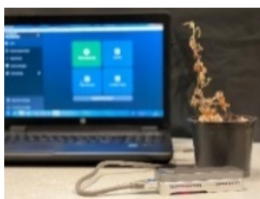
Fig. 1: Using MinION for plant virus/viroid detection.
