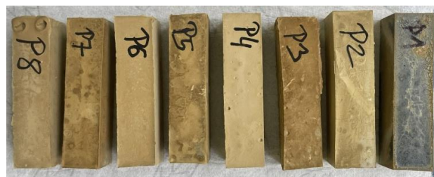
Figure 1: Alkali activated materials prepared of different alternative activators.
