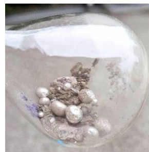
Figure 1: Collected sodium in a flask
