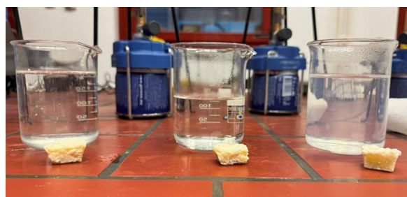
Figure 1: Condition of squares made from different types of milk after the endurance test
