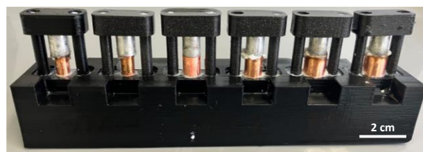
Figure 1: An example of galvanically coupled AA6082 and Cu-ETP mounted in 3D printed holder during testing in the salt spray chamber (after 192 hours).
