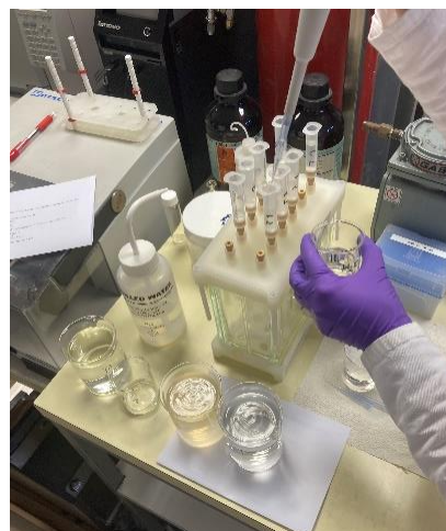
Figure 1: Solid-phase extraction cartridges (Oasis MCX) used for sample concentration from wastewater samples collected in Ljubljana and Trbovlje.
